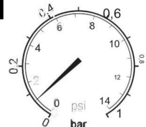
Now the lower chamber can be inflated. The air pressure pumped into the lower chamber must be min. 0.2 psi / 0.01 bar or max. 0.8 psi / 0.05 bar. The ideal pressure at the bottom is 0.5 psi / 0.03 bar. Make sure that the valve cover lock is closed after inflation.
